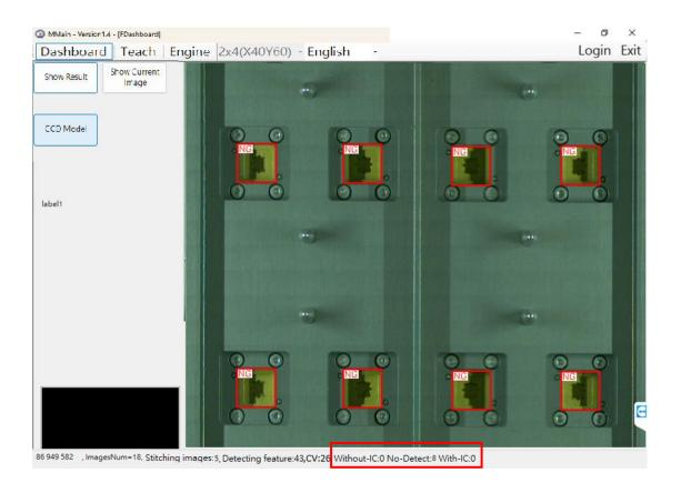
If "Without-IC" is inconsistent, decrease the Matching Ratio and move the shuttle again until the "Without-IC" count in the status bar below matches the DUT.
