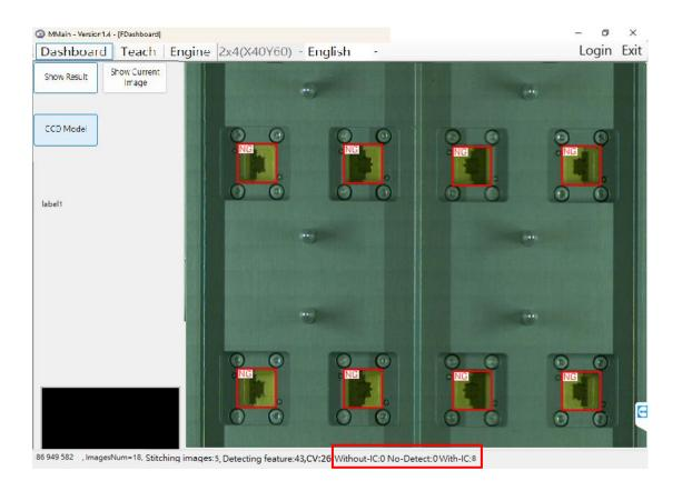
If "Without-IC" is inconsistent, increase the Color Difference and move the shuttle again until the "Without-IC" count in the status bar below matches the DUT.
