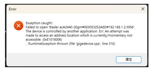
Indicates that another application is currently connected to the CCD hardware. You can restart the CCD network and reconnect.
