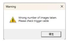
Determine if there is a trigger line anomaly based on the number of images taken. If the count is zero or if an incorrect number of images is taken, this warning window will be displayed. Please refer to the Engine page.
